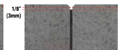
PAVERS OR NATURAL STONES WITH CHAMFER
